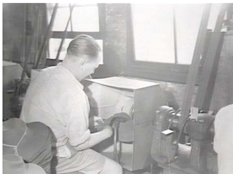
Figure 5.3.3 Skilled machinist preparing a felt hat by machine sanding the brim and crown. Note the overhead belt driven machinery in this part of the factory (possibly Nos. 7-9). March 1949
